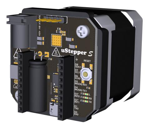
The super slim design of **uStepper** *S* makes it possible to develop applications using a stepper motor, without the need for long and messy wiring to an external Arduino/stepper shield. Furthermore the 16-bit rotary encoder ensures that the absolute position of the motor shaft can be tracked, enabling the **uStepper** *S* to detect any loss of steps and act on it !
