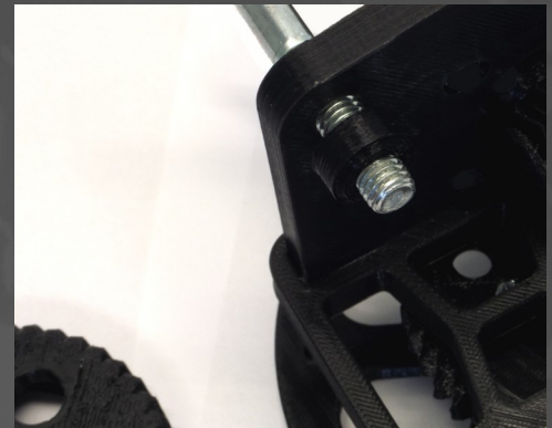
Fig.16: Insert the M8x70 mm bolt in the left side plate (14) and add the short M8 spacer (32).
