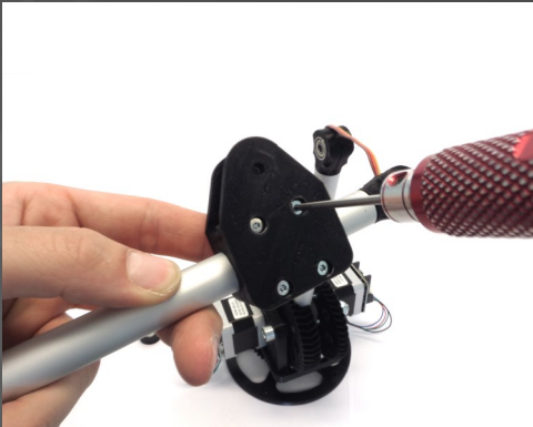
Fig.37: Mount the main joint bracket ⑦ and ⑧ on the longer tube. The position of the tube in the bracket is adjusted in the final step.
