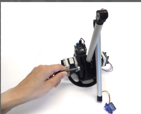
Fig.35: Add an M8 SL nut on the right side and tighten the bolt. (Do not overtighten)
