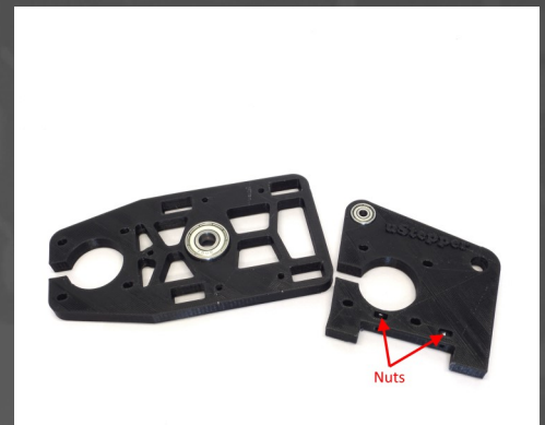
Fig.4: Fit a 608Z bearing in the bottom plate (13), a 624Z bearing and two M3 nuts in the side left plate (14).
