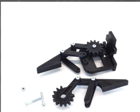
Fig.51: Mount the gear to the bracket from fig. 48 as shown, using an M3x20 mm bolt and an M3 SL nut. (Make sure the parts move freely)
