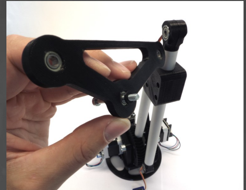
Fig.38: Add 3 624Z bearings to the triangle ⑨, add an M4x35 mm bolt and the short M4 spacer ⑩.
