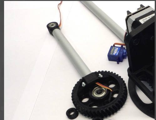
Fig.32: Slide the short 15 mm tube into the main gear (4) and secure it with the bracket (5) using 2 M3x20 mm bolts and 2 M3 nuts.
