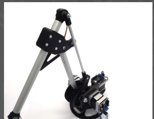
Fig.42: Mount one of the two 169 mm arms (tube length) as shown. Requires 1 M4x20 mm and 1 M4x35 mm bolt and 2 M4 SL nuts.
