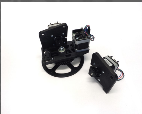
Fig.23: This is how the assembly should look by now. With the gear and M8 bolt removed.
