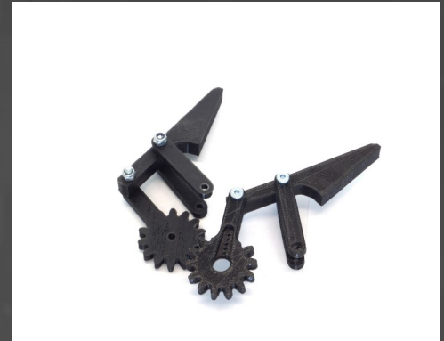
Fig.50: Use 4 M3x20 mm bolts and 4 M3 SL nuts to assemble the parts as shown above. (Make sure the parts move freely)
