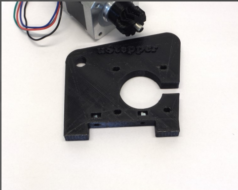
Fig.19: Insert 2 M3 nuts in the right side plate (15).
