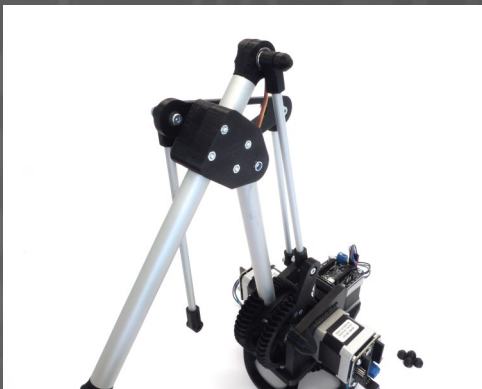
Fig.45: Add the M8 nut cover (25) and the longer M4 nut cover (27) as shown.
