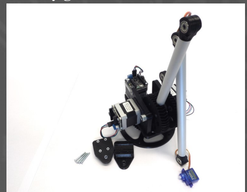
Fig.36: Add 4 M3 nuts and 1 M4 SL nut to the main joint bracket (7) and (8) as shown. Prepare 4 M3x25 mm bolts for assembly.
