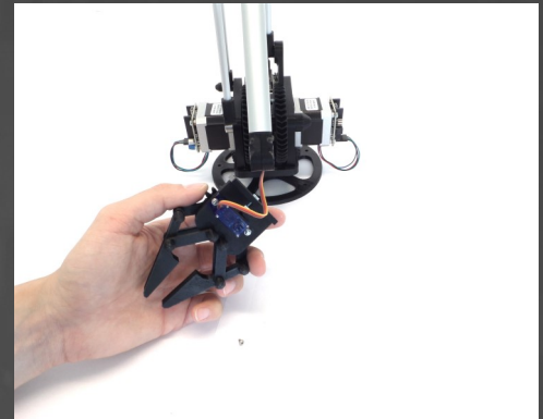
Fig.56: Use the two longer screws from the servo accessories bag to mount the servo.
