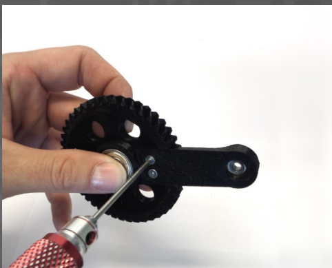
Fig.21: Fit a 624Z bearing in the second gear arm (6), and attach it to the secondary gear (3) using 2 M3x10 mm and 2 M3 nuts
