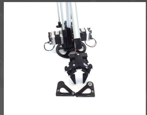
Fig.58: Add a 624Z bearing to the left end triangle (17) and an M4 SL nut to the right (16).
