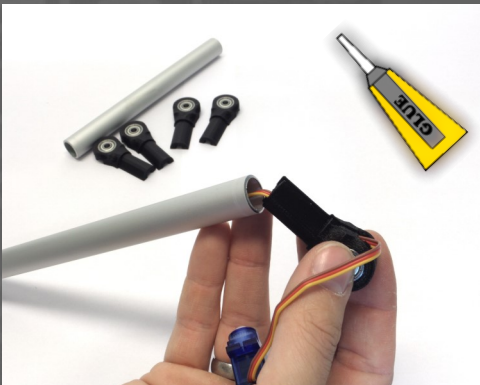
Fig.29: Insert the servo cable prior to insertion of the rod ends (10) and (11) into the tube.
