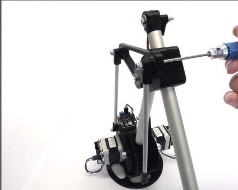
Fig.43: Mount the other 169 mm link arm from side plate to triangle and the 164 mm link arm as shown. Use 3 M4x20mm bolts and 3 M4 SL nuts.
