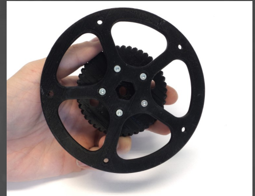
Fig.2: Assemble base (1) and base gear (2) using 5 M3x25 mm bolts and 5 M3 nuts.
