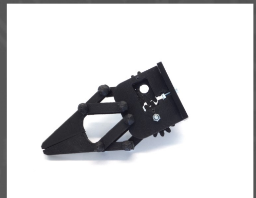
Fig.54: Add M3 nut covers 28 to all nuts but the one holding the gear, as shown here.
