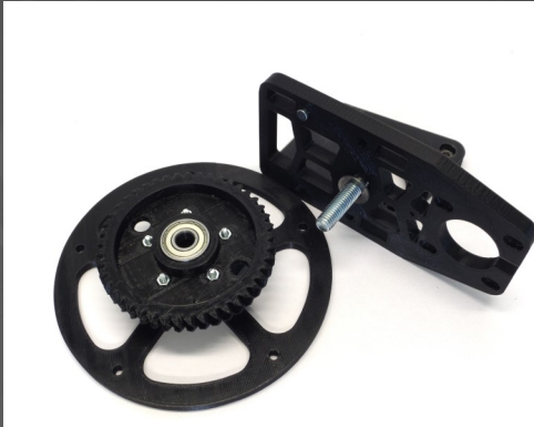
Fig.7: Insert the M8x40 bolt in the bottom plate (13), and add a washer. Place an M8 SL nut in the base (1) (not visible here, see fig. 11)
