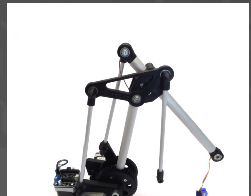
Fig.46: Add the 4 M4 nut covers (26) as shown.
