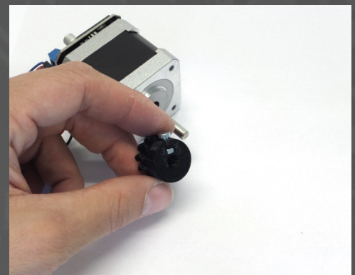
Fig.18: Insert nut and M3x8 mm bolt in the secondary motor gear (3).
