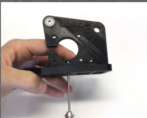
Fig.5: Press the left side plate (14) into the bottom plate (13) without using excessive force. Secure it using 2 M3x10 bolts.
