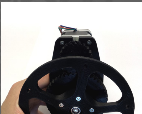
Fig.11: Mount the motor and motor gear (2). Secure the motor to the bottom plate (13) using 4 M3x10 mm bolts.
