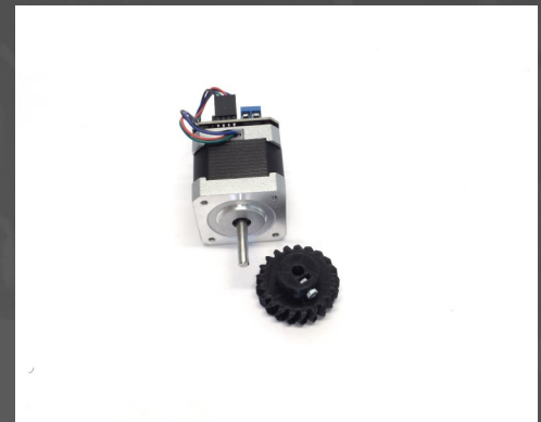
Fig.10: Insert an M3 nut and an M3x8 mm bolt into the base motor gear (2).
