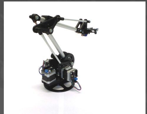
Fig.64: Adjust the position of the tube as mentioned in fig. 37 so that the gripper is level with the base.
