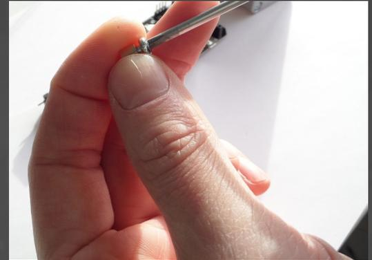
Fig.2: Insert mounting screw into stand-off.
