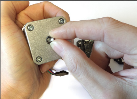
Fig.3: Drop in the encoder magnet.
